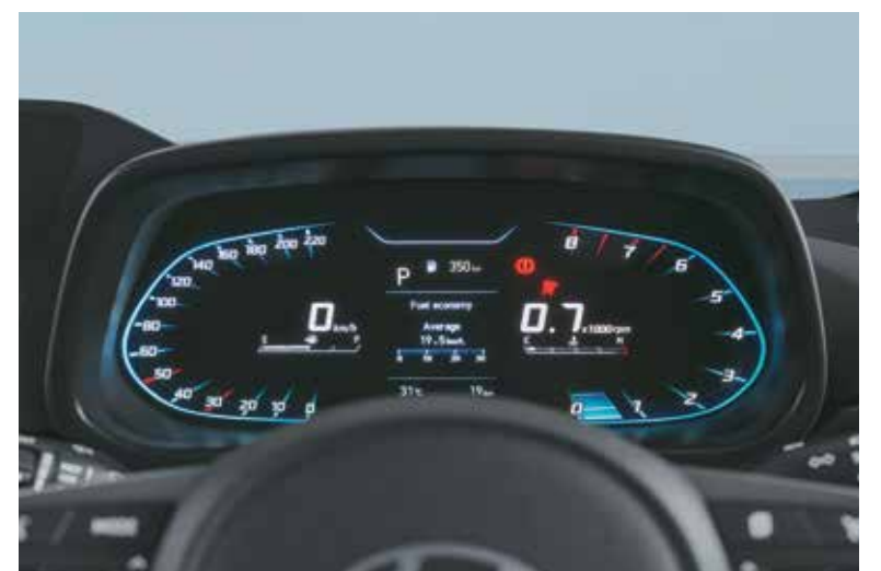
Digital cluster with TFT multi information display
