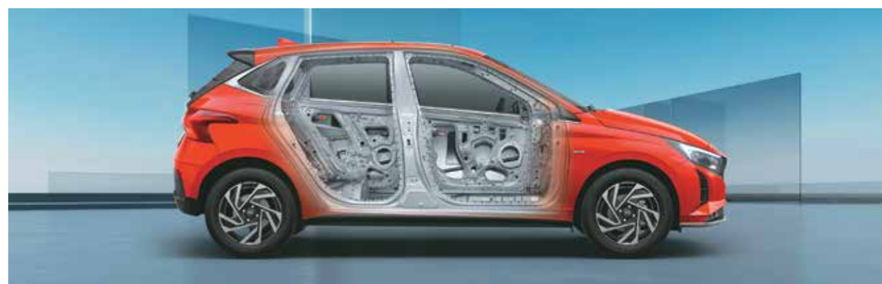
Strong body structure (with AHSS and HSS)
